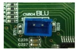
There are two blue terminals on the outdoor control panel, as shown above. Application: Short out the terminals, and power up the outdoor unit, then the outdoor unit may run independently. It can be determined that there is no internal and external communication faults.
