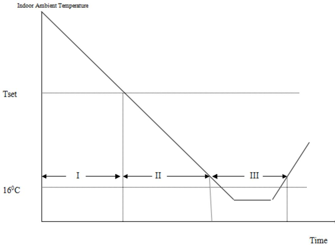
Dehumidifying area I: Operation at the frequency in the range (30–60Hz) according to  $Dt$  ( $T_{\text{indoor ambient}} - T_{\text{set}}$ ).
