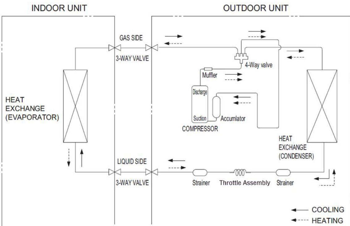
NOTE: In different models, the throttle assembly may be Capillary or Electronic expansion valve.
