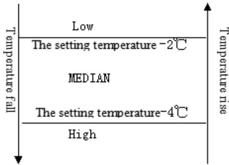
When the difference between the setting temperature and the room temperature equal to 2°C or 4°C, the indoor fan speed will keep in current speed.
