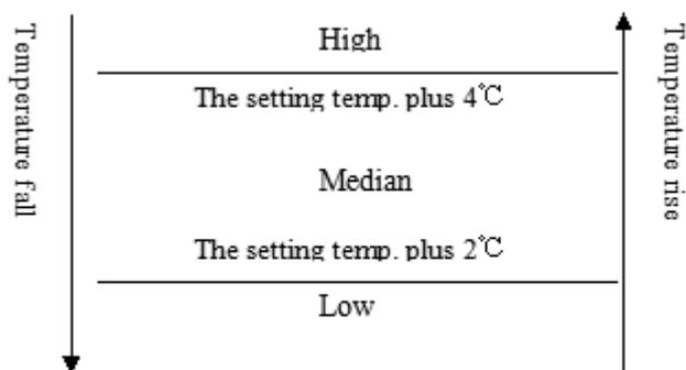
When the difference between the setting temperature and the room temperature equal to 2°C or 4°C, the indoor fan speed will keep in current speed.
