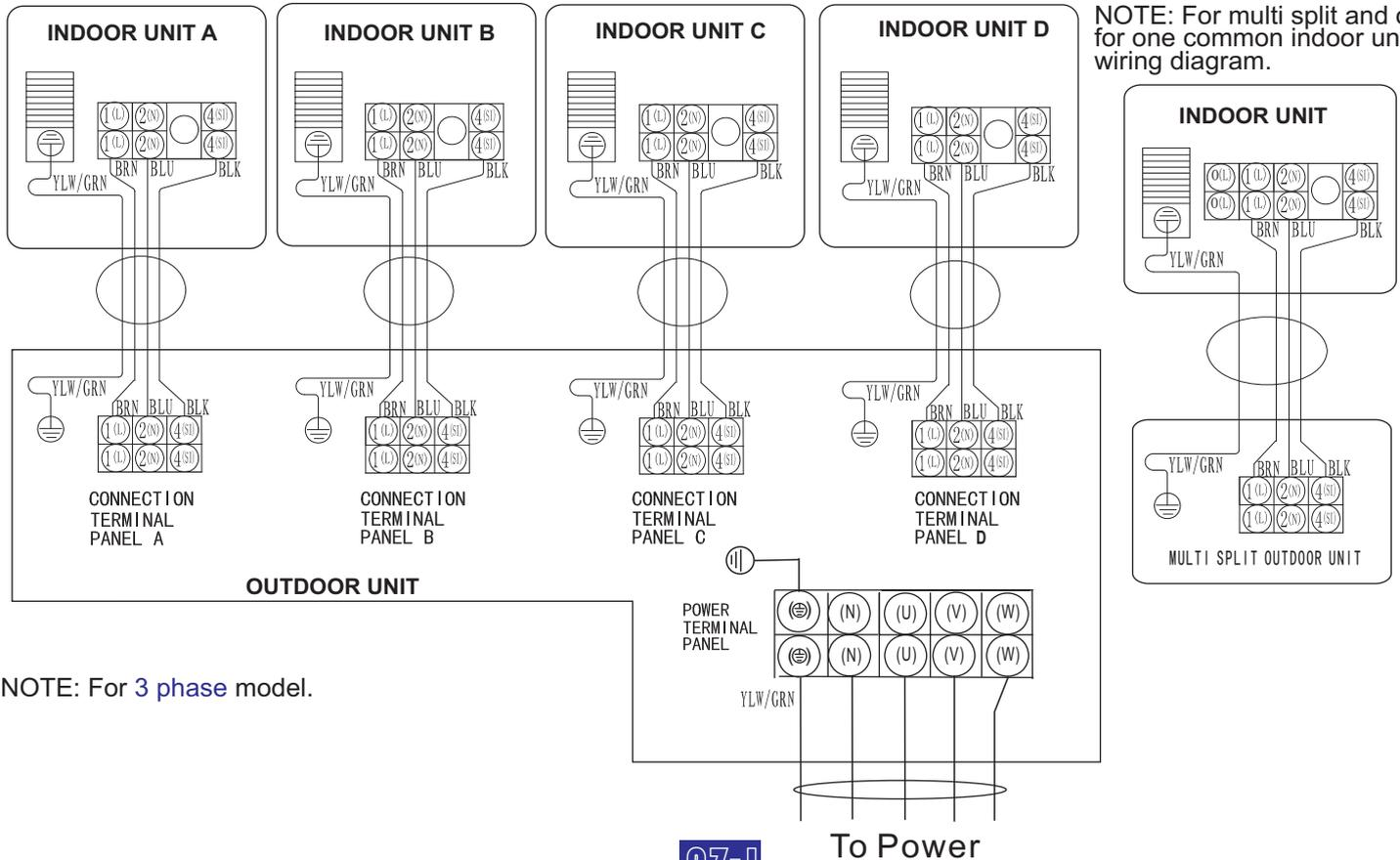
NOTE: For multi split and one for one common indoor unit the wiring diagram.
