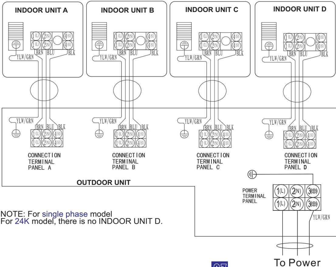
NOTE: For multi split and one for one common indoor unit the wiring diagram.
