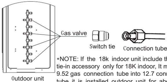
\*NOTE: If the 18k indoor unit include the switch tie-in accessory only for 18K indoor, It may switch 9.52 gas connection tube into 12.7 connection tube, it is installed outdoor unit for above Picture.
